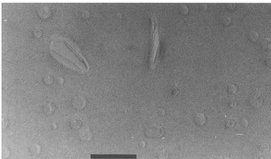
Fig. 2. TEM picture of CA particles prepared by precipitation in an emulsion system. The CA concentration was 25% (w/w) in cyclohexane and the surfactants were phosphatidylcholine and sodium glycocholate. Bar: 100 nm.
